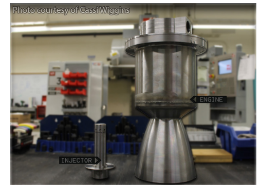
The image above is the bench-test engine, "which is quite heavy and a little overbuilt for safety's sake, but does resemble the flight design," Hirsh said.
