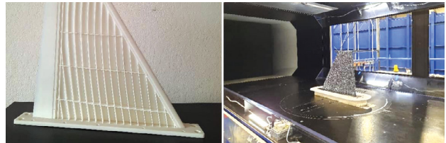
Left: 3D printed wing model without lower skin attached. Right: The wing mounted inside the wind tunnel test section.
