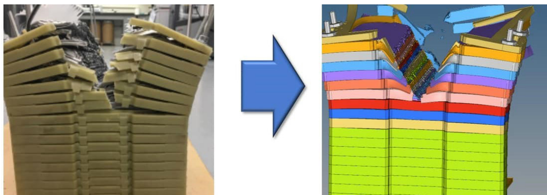
These side-by-side images show a lithium-ion battery failure following a laboratory test, compared with a computer simulation of the event. (Photo courtesy of Dr. Zhu)
